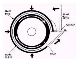
This is a very simple type of brake using the principle that a band is wrapped part round a rotating drum. Tension can be applied to the band using a lever. The restraining torque results from the difference in tension between the two ends of the belt.
